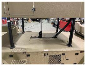
Before each use of the Cabra, always make sure the hydraulic hose going into the hydraulic rams is free to move and that there is no chafing. There is a safety hose burst valve installed on the rams so that if the hydraulic hose breaks the valve closes and the cab will not come down. The only way to get the cab to come down in that event is to restore hydraulic pressure to the hydraulic rams.
